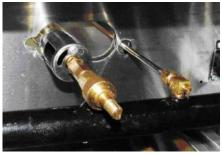
3. Replace the orifice fittings into the valve.
